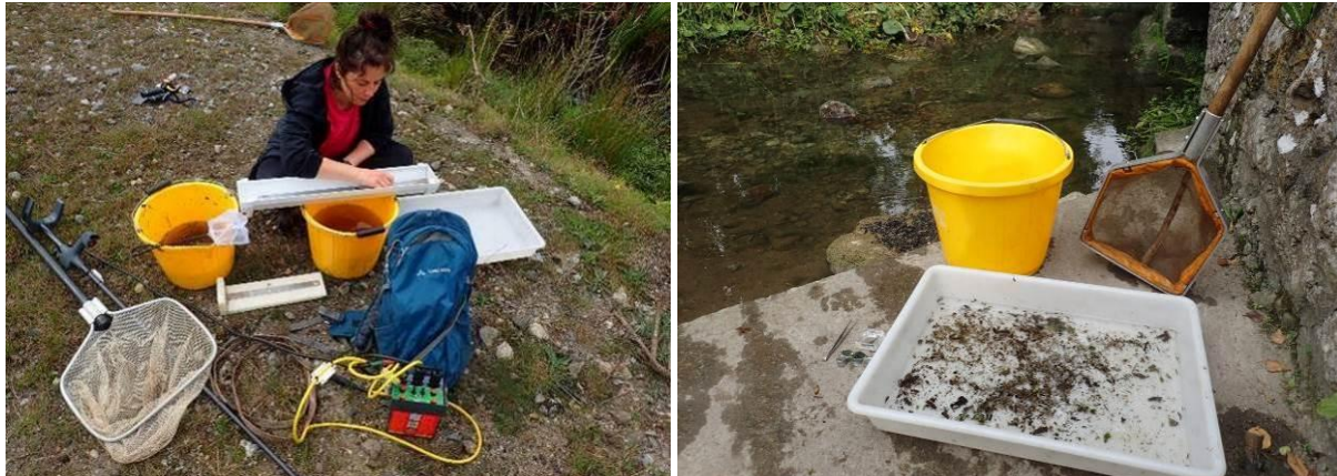
Plate 2.1: Electrical fishing sampling apparatus employed during the on-site investigations (left). Macroinvertebrate sampling kit used during biological water quality assessment (right)
